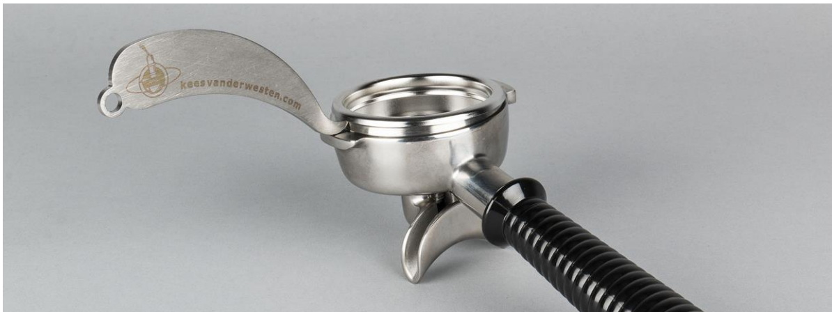
Figure U 6. Pry filter basket from filter holder with the group screen extractor.
