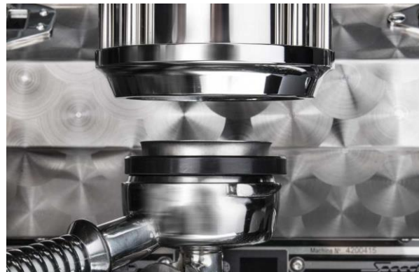
Figure U 7a (left). Gently pry left and right with group screen extractor to remove group screen and group seal.
