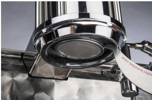
Figure U 7a (left). Gently pry left and right with group screen extractor to remove group screen and group seal.
